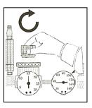
**Note:** The higher the pressure on the 0-30 gauge, the larger the insecticide particles will be. A higher pressure will be required when working overhead (above 6-8 ft.) to compensate for the effects of gravity. Adjust in 1 or 2 lb. increments to achieve desired flow and particle size.
