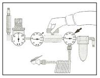
To use the air chuck the compressor must be running. Turn the handle of the ball valve, located on the manifold, in the cross line position. The adjustable 100 psi relief valve will relieve at 70 psi and will produce a notable popping sound.
