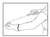
E. Holding the wand over the tank, place gloved finger over integrated stainless crack & crevice tip exit orifice, stopping the flow of air, then squeeze the application trigger until liquid is purged from the wand and hose.
