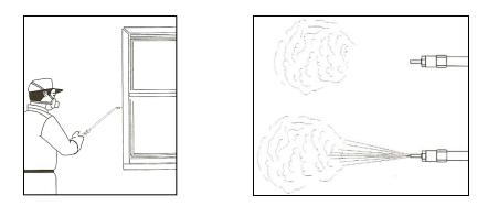
**Helpful Hints:** Occasionally, when working overhead, the pressure exerted on the liquid tank by the regulator will not be sufficient to drive the liquid 8-10 feet above floor level. At this time, you need to increase the pressure on the liquid tank by adjusting the regulator clockwise to the point you receive the aerosol at the tip and at the height you desire to work. When returning to ground level be sure to adjust regulator back to normal operating pressure.
