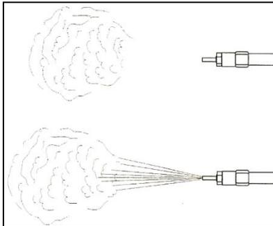
**Helpful Hints:** Occasionally, when working overhead, the pressure exerted on the liquid tank by the regulator will not be sufficient to drive the liquid 8-10 feet above floor level. At this time, you need to increase the pressure on the liquid tank by adjusting the regulator clockwise to the point you receive the aerosol at the tip and at the height you desire to work. When returning to ground level be sure to adjust regulator back to normal operating pressure.
