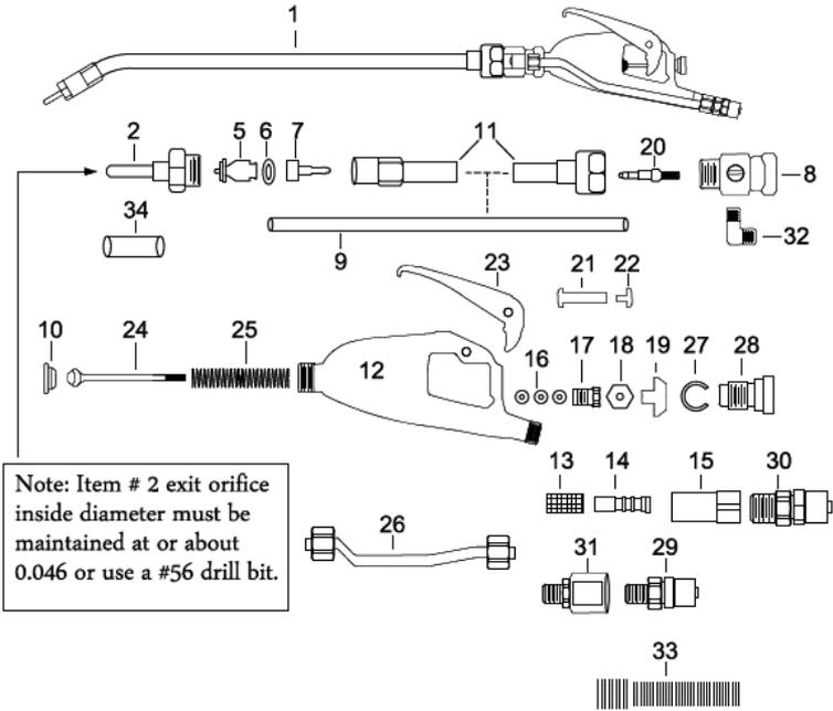
Note: Item # 2 exit orifice inside diameter must be maintained at or about 0.046 or use a #56 drill bit.
