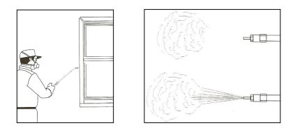
**Helpful Hints:** Occasionally, when working overhead, the pressure exerted on the liquid tank by the regulator will not be sufficient to drive the liquid 8-10 feet above floor level. At this time, you need to increase the pressure on the liquid tank by adjusting the regulator clockwise to the point you receive the aerosol at the tip and at the height you desire to work. When returning to ground level be sure to adjust regulator back to normal operating pressure.
